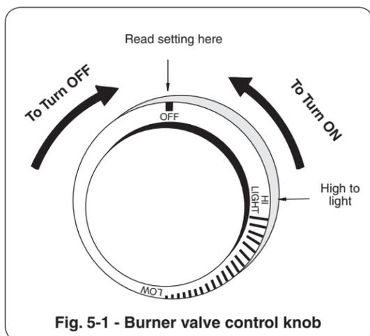
Fig. 5-1 - Burner valve control knob
