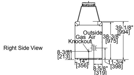
Framing dimensions in illustrations accommodate 1/2" finishing material.
