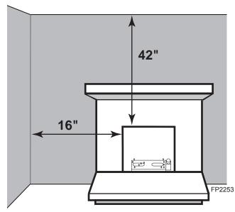
Figure 3 - Sidewall and Ceiling Clearances
