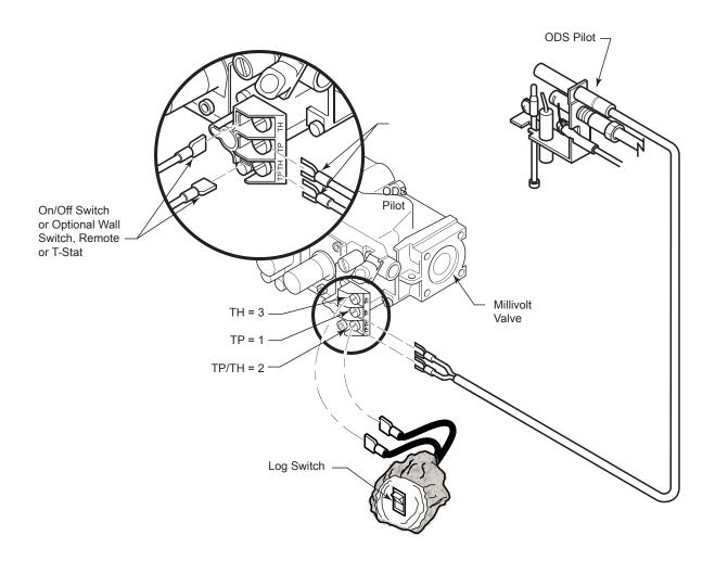
Figure 16 -Wiring Diagram
