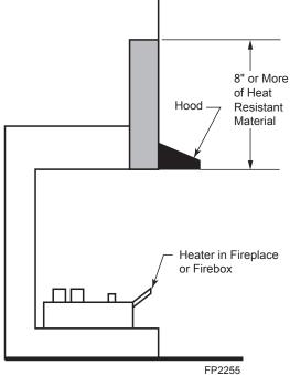
Figure 5 - Measuring Heat Resistant Material for Mantel
