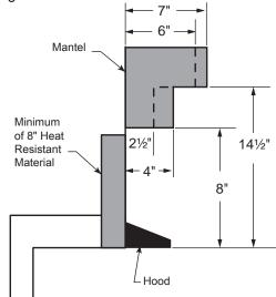
Figure 9 - Minimum Mantel Clearance with Hood — NB24 (Example of Unsafe Installation)
