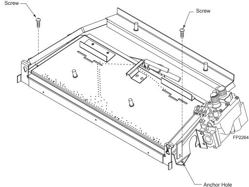
Figure 13 -Securing Heater to Floor of Fireplace/Firebox
