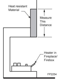
Figure 4 - Measure Heat Resistant Material
