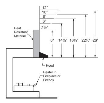
Figure 7 - Minimum Mantel Clearance with Hood — All Models
