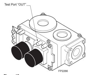
Figure 15 -Pressure Test Point Location Millivolt Control
