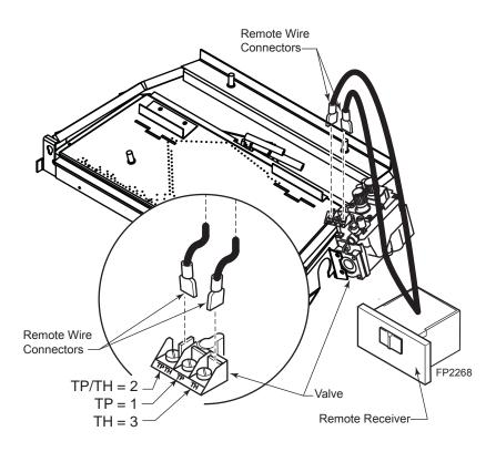
Figure 17 -Installing Remote Receiver
