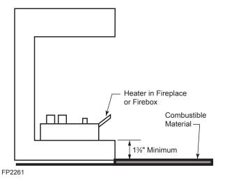
Figure 10 - Minimum Clearance above Combustible Flooring
