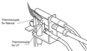
Figure 43 - Correct Appearance of Pilot Flame
