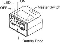
Figure 48 - Signature Command System Components
