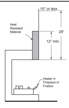
Figure 8 - Minimum Mantel Clearance with No Hood — NB24
