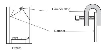
Figure 12 - Damper Stop Installation.
