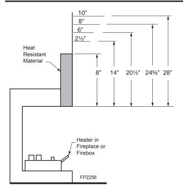
Figure 6 Minimum Mantel Clearance with No Hood — NB18
