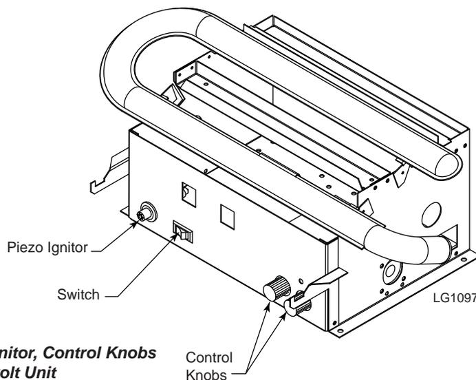
**Location of Piezo Ignitor, Control Knobs and Switch on Millivolt Unit**
