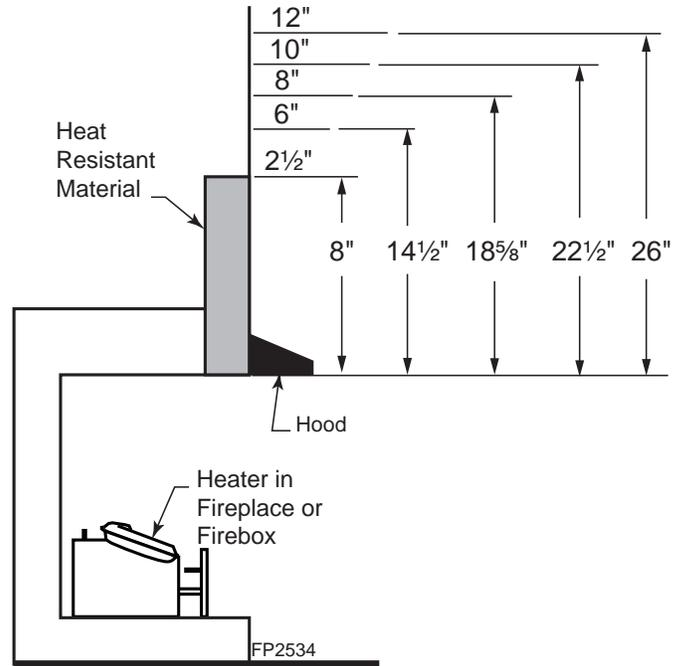
Figure 6 - Minimum Mantel Clearance with Hood
