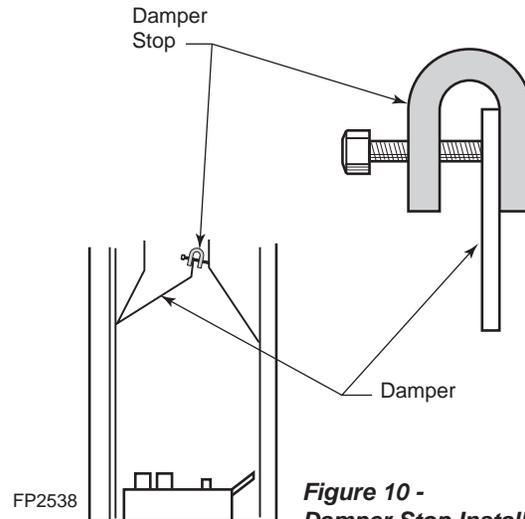
**Figure 10 - Damper Stop Installation (See Warning)**
