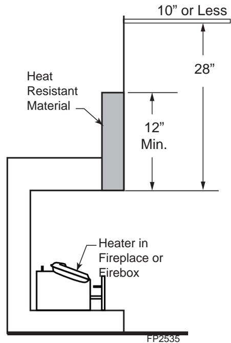
Figure 7 - Minimum Mantel Clearance with No Hood
