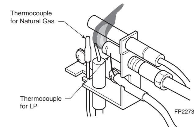
**Figure 29 - Incorrect Pilot Flame Appearance**
