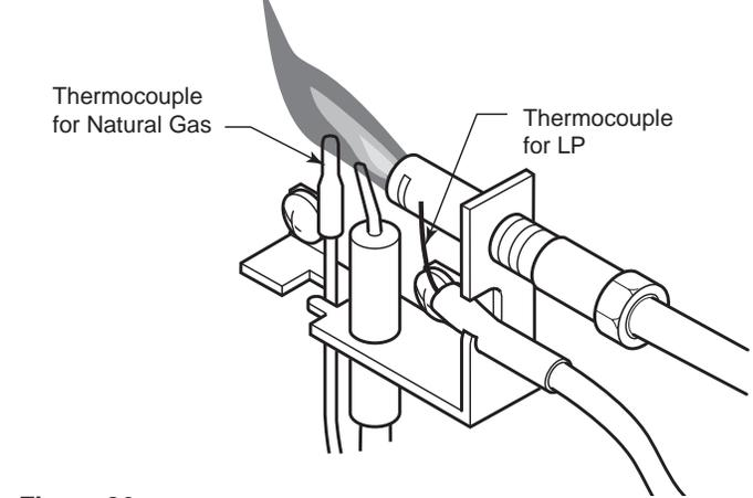
**Figure 30 - Correct Pilot Flame Appearance**
