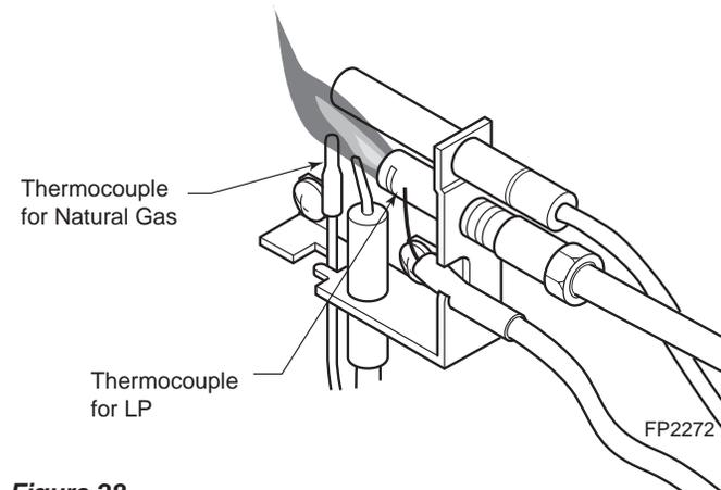
**Figure 28 - Correct Pilot Flame Appearance**
