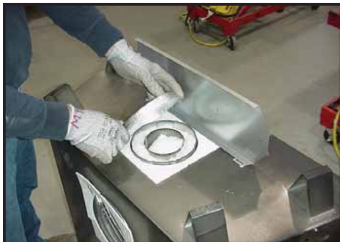
Figure 6.5 Remove the seal cap.
