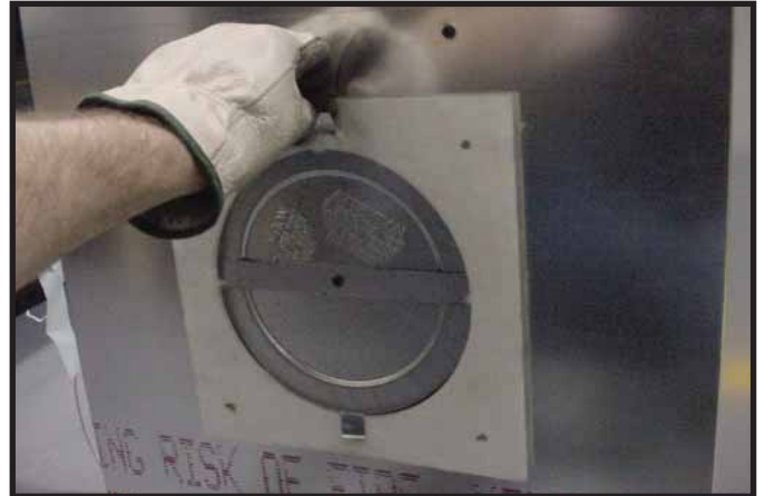
Figure 6.9 Fold the tabs toward the center of the fire plug (90°) and remove the insulation gasket.
